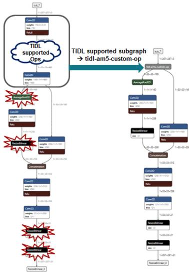
Fig. 4 Original and TIDL compiled Deeplab v3 TFLite model.
