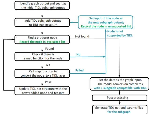
Fig. 3: TIDL import execution flow with enhancement for subgraph partitioning (marked in bold and in blue/green color).
