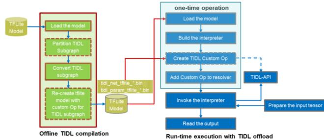
Fig. 2: Framework for TFLite heterogeneous execution with TIDL.
