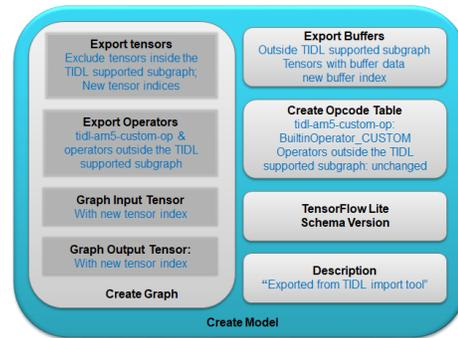
Fig. 5 Serialization to create the output model in FlatBuffers format.
