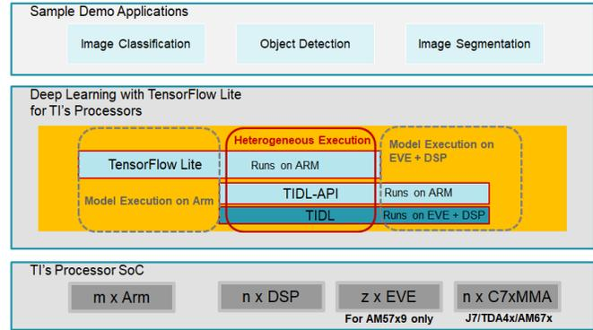
Fig. 1 Deep learning with TFLite for TI's processors: Arm only, TIDL only, and heterogeneous execution.
