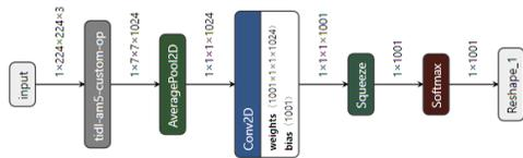
Fig. 8: Compile mobilenet v1 model for heterogeneous execution.
